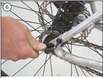
Tighten the two drive side bolts so that they're fixed, but not torqued to specification yet.
